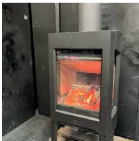
The stove on the test rig, output test
