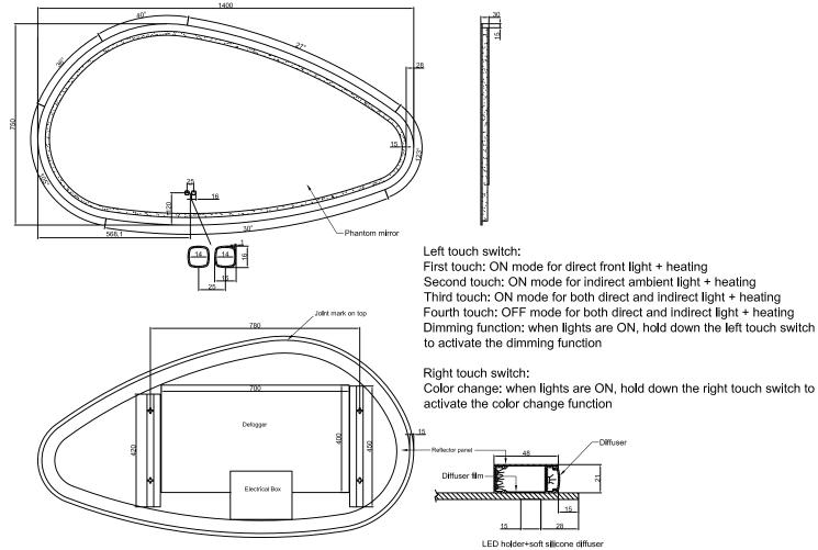
Phantom mirror model 7 Size:W1400\*H750mm Front LED Light: 2835/24V/360pcs/2700~6400K/54W LED Length:3.1m Backlit LED Ligh: 2835/24V/120PCS/20W/2700K~6400K LED Length:3.4m Heating film: 700\*400mm
