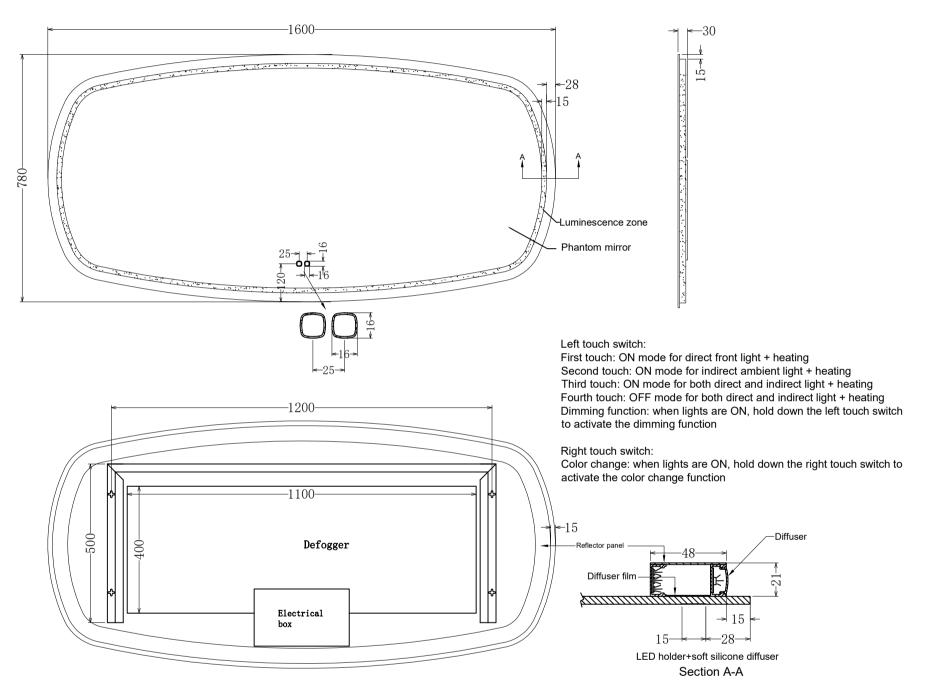
007.160.78 Size:W1600\*H780mm Front LED Light: 2835/24V/360pcs/2700~6400K/54W LED Length:3.8m Backlit LED Ligh: 2835/24V/120PCS/20W/2700K~6400K LED Length:4.0m Heating film: 1100\*400mm CE IP44
