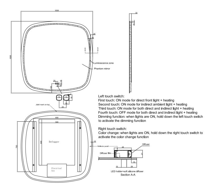
Phantom mirror model 5 Size:W1000\*H1000mm Front LED Light: 2835/24V/360pcs/2700~6400K/54W LED Length:3.05m Backlit LED Ligh: 2835/24V/120PCS/20W/2700K~6400K LED Length:3.3m Heating film: 640\*500mm CE IP44
