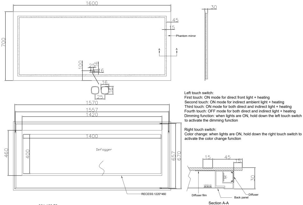
001.160.70 Size: 1600\*700H Front LED Light: 2835/24V/360pcs/2700~6400K/54W LED Length:4.2m Backlit LED Light: 2835/24V/120PCS/16W/2700K~6400K LED Length:4.4m Heating film: 1400\*400 CE IP44
